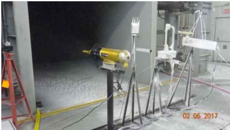
Figure 1: Microphysical sensors in the CWT from left to right used in the analysis; GCIP probe (10-960 micron), WXT, LPM (100 micron-1 cm), and Gondola sensors that include CDP (2-50 micron) and BCP sensors (5-100 micron).
