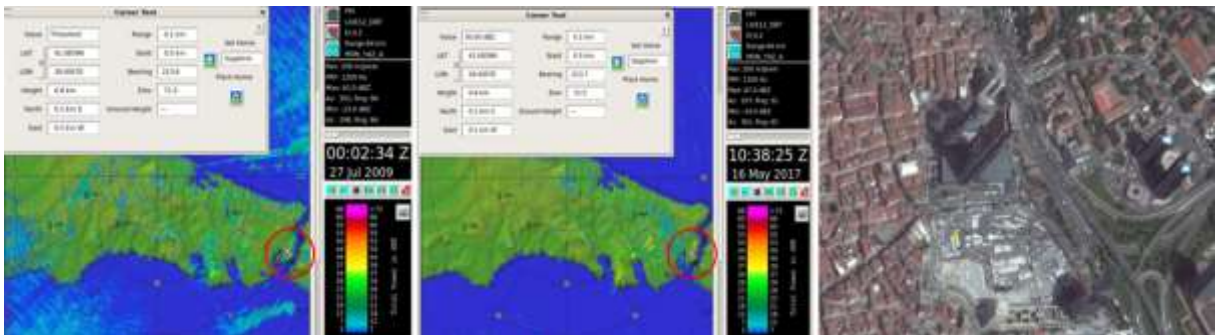
Figure 9. The comparison of PPI dBZ products in 2009 and 2017. Corresponding coordinate in Google Maps shows Sapphire Skyscraper location
