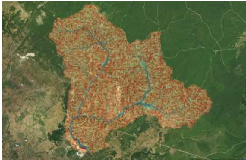
Figure 3. Topographic wetness index map using low resolution DEM data.
