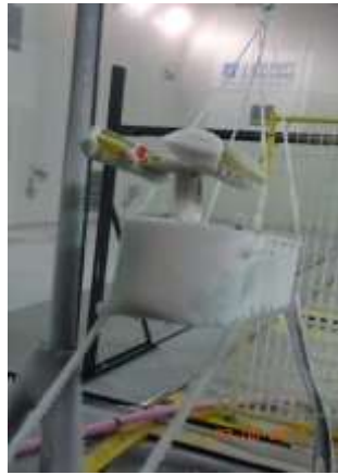
Figure 6: Icing occurred on Aug 26 2016 case on the Gondola platform.
