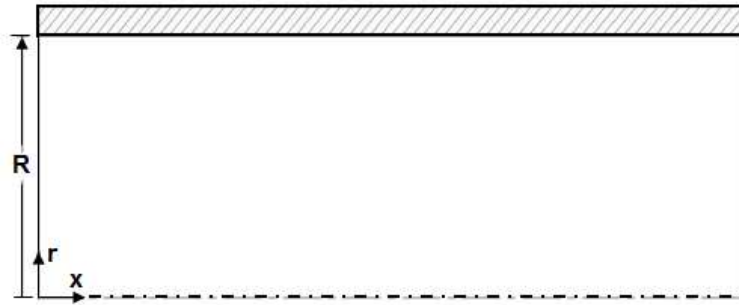
Figure 1. Axisymmetric cylindrical coordinate system and geometry of the pipe flow.
